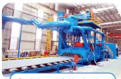
Semi-automatic blasting shop
